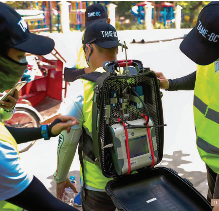
01 Using a mobile backpack Aethalometer, Quezon City team roams the streets to determine levels of Black Carbon in the air
